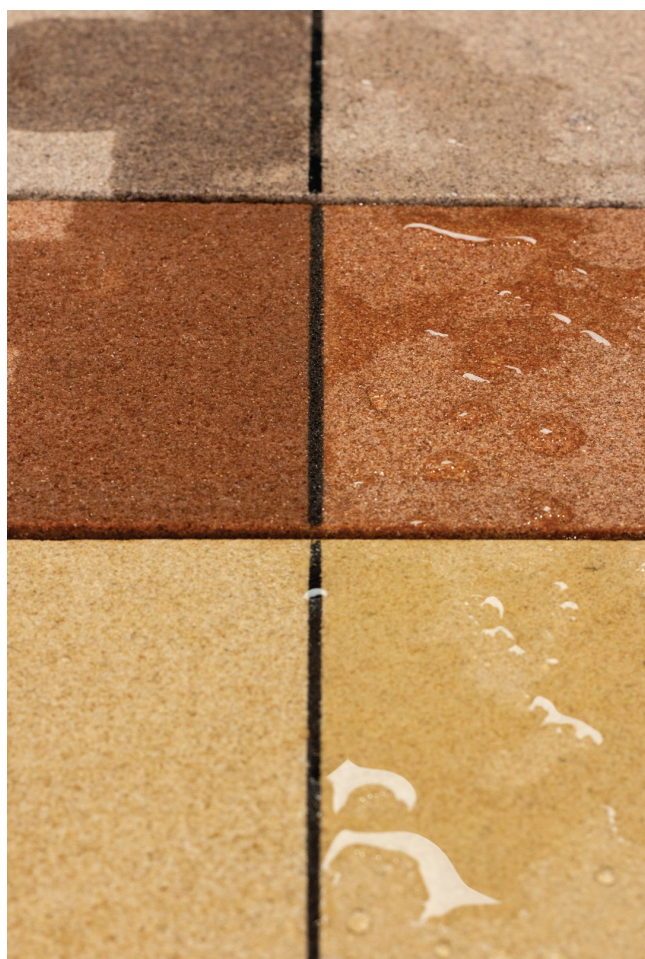
Water applied to a natural stone tile treated with a non-breathable sealer on the right compared to an untreated sandstone tile on the left.
